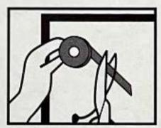
2). Cut lengths needed form roll. Do not remove protective liner as yet.
