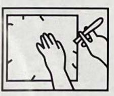
1). Make light pencil lines on wall at key. Points around object to be mounted.
