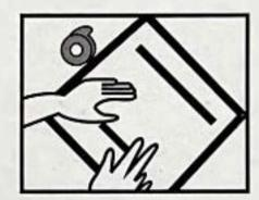
3). Press tape into position on back of object to be mounted. Press firmly on liner for good adhesive contact.
