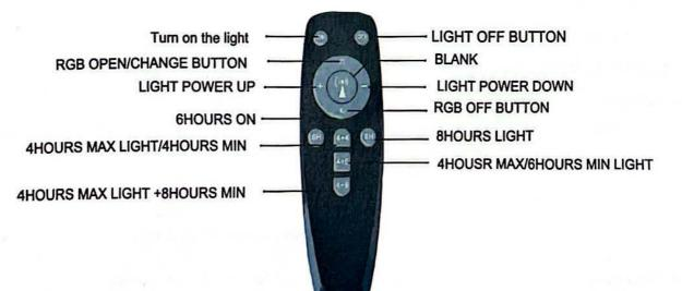
**Note:** once the ON/OFF button is pressed, the light control is colsed. If you want to switch on in the evening. You need to press the AUTO button to activate the light. Otherwise solar panels will not start lighting at night auomatically
